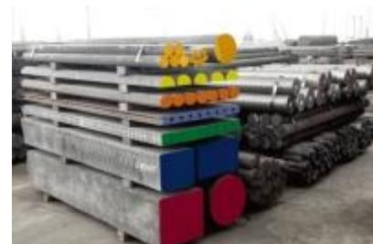
**Territoire d'innovation / Area of innovation :** H-BAR ductile iron can be used as an alternative to medium carbon steel, with similar strength, but ductile iron has better machinability.
